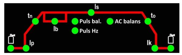
Gas bottle symbol - Adjustment of a shield gas supply before arc ignition
